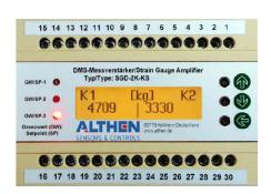
This programmable dual channel strain gauge amplifier offers supply and signal evaluation for two strain gauge transducers. With the respective setting this amplifier can be used for differentiation, for summation or for displaying one or both channels. Furthermore 3 programmable limit switches (potential free relay contacts max. 30 V, 0.5 A) can be set over the total measuring range. For further analysis a 4 ... 20 mA analogue output signal is available.
