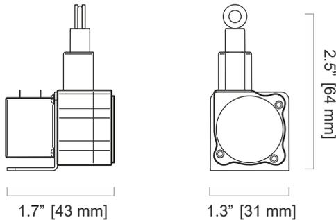
With its ultra compact design the SM1 is the perfect solution when tight space is an issue. At just a little over an inch across, this miniature stringpot offers full stroke measurement ranges from 2.4 to 25 inches. A precision plastic hybrid 10K-ohm potentiometer delivers a precise voltage divider output signal that is linearly proportional to the travel of the spring-loaded measuring cable.
