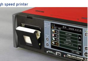
High speed thermal printer is integrated. Its printing speed is 0.04 seconds for one line of one channel. Applicable paper: P-80 (80 mm wide)
