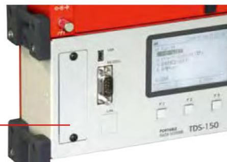
Switching box/TML-NET driving board
