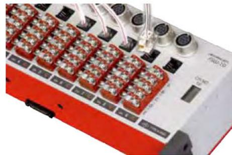
**TML-NET for 2-wire digital network measurement**
