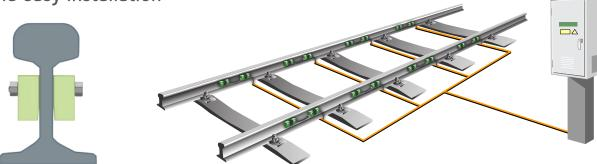
Our patented bolt-on sensors do not require the track to be closed during installation and maintenance which dramatically reduces traffic interferences. The sensors need to bolted in place either through holes or using our weldable sockets.
