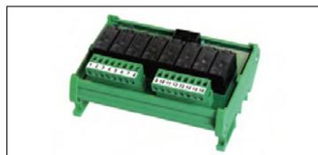
External 8-relay module to manage from 7 to 14 product; to be added to RELE6PROD module; 8 relays up to max. 115VAC/2A. already included for mod. 14 PRODUCTS.
