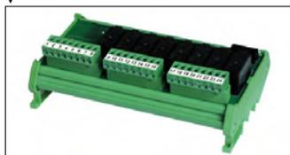
External 8-relay module to manage from 1 to 6 products; 8 relays up to max 115VAC/2A. Module already included for mod. 6/14 PRODUCTS.
