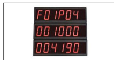
Manual batching with remote displays (example of application with 3 remote display side by side). This option allows to display on different remote displays, connected in parallel to the instrument via RS485 serial port, the following batching information: formula and product number, instrument status, the remaining quantity to be batched, gross weight.
