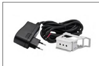
24VDC 1A stabilized power supply, input 100-240 VAC, 3 meters long cable, with socket and support for Omega rail.
