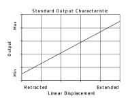
**Output Characteristic:** Target is extended 7 mm from end of body at start of normal travel. The output increases as the target extends from the sensor body, the calibrated stroke is between 5 mm and 800 mm.
