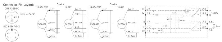
**Putting Into Service:** The sensor must be used with a galvanic isolation barrier designed to supply the sensor with a nominal 5V and to transmit the sensor output to a safe area.
