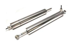
This intrinsically safe X114 LIPS® (Linear Inductive Position Sensor) is an affordable, durable, high-accuracy position sensor derived from the X101. Designed for applications where the sensor would be completely submerged during normal operation, it retains desirable features such as compact size, good sensor performance yet capable of working in pressures up to 10 bar.
