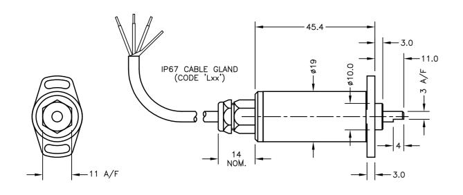
FLANGE BASE (STANDARD) 2 OFF 3.2 SLOTS ±15° ON 25.0 PCD. (SYMMETRICAL)
