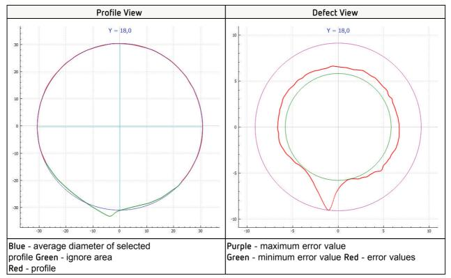
To view the profile deviations in depth, tick the DEFECT VIEW box in the toolbar.
