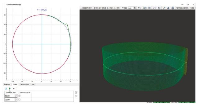
To select a profile to view in the Profile View mode, hold the Ctrl key pressed and click the left mouse key on the profile. In the 3D View mode, the selected profile will be highlighted.
