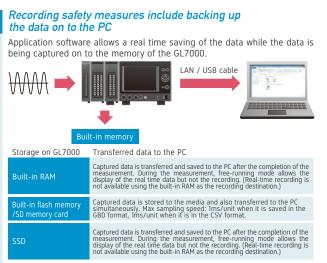
Peal time recording on the PC can be saved as a CSV file while the data is saved as a GBD file on the main GL7000. Maximum sampling speed for this feature is Ims.
