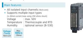
Supports one humidity sensor per module (B-530). Additional humidity sensors require an external power supply for the sensors.
