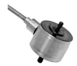
Model 31E low range precision miniature load cells measure both tension and compression load forces of 0.5 N to 5 N. These models are our highest accuracy, rugged miniature load cells. Model 31E's welded, stainless steel construction is designed to eliminate or reduce to a minimum, the effects of off-axis loads. (The internal construction assures excellent long-term stability for ranges 1000 grams and above.)
