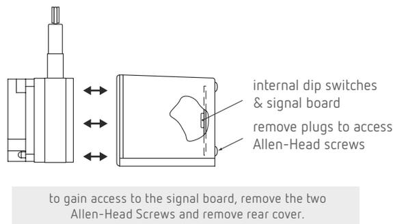
The output signal direction can be reversed at any time by simply changing the dip-switch settings found on the internal signal board. After the settings have been changed, adjustment of the Zero and Span trimpots will be required to precisely match signal values to the beginning and end points of the stroke.
