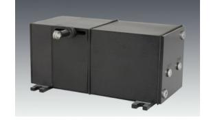
The PT5AV is a combination position and velocity trans- ducer. A precision plastic-hybrid potentiometer provides accurate position feedback while a self-generating DC tachometer provides a velocity signal that is proportional to the speed of the traveling measuring cable.
