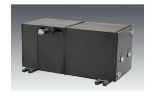
The PT5CN cable extension position transducer communicates linear position via the CANbus SAE J1939 interface providing a precision position feedback to your PLC. The PT5DN is offered in full stroke ranges up to 250 inches and a thermoplastic measuring cable for high cycle and rugged applications.
