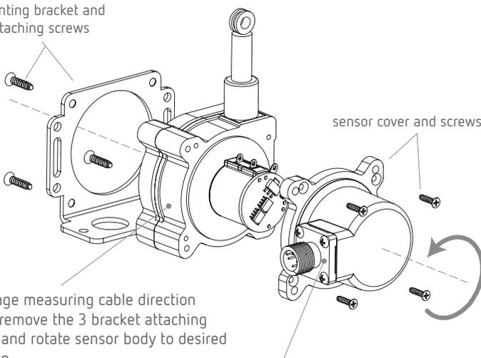
To change measuring cable direction simply remove the 3 bracket attaching screws and rotate sensor body to desired direction.
