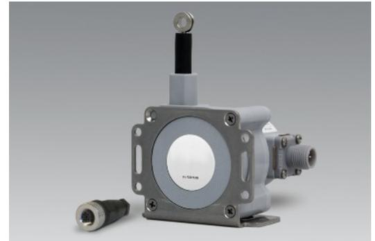
This compact stringpot provides the ultimate in ease-of-use and flexibility. This sensor fits in small spaces, doesn't need perfect alignment, mounts in just about any direction imaginable and has a unique circuit that lets the user choose 4-20mA or 0-10Vdc output on the fly.
