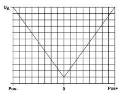
between these two voltages. This output signal is, depending on the direction the core moves, either in phase or 180° shifted to the excitation voltage. When the core is in central position between the two secondary coils the 2 voltages cancel each other out, except for a small voltage will always be there due to minor asymmetries.
